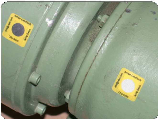
JUMBO-CelsiDot® with one level at 93°C. Left CDJ exceeded sometime in the past its 93°C level. CDJ to the right not heated.
